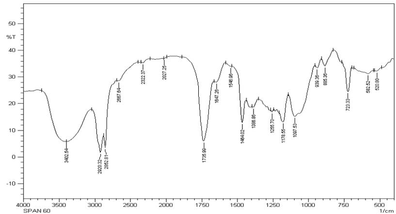
Figure no.3: IR spectrum of Span60
