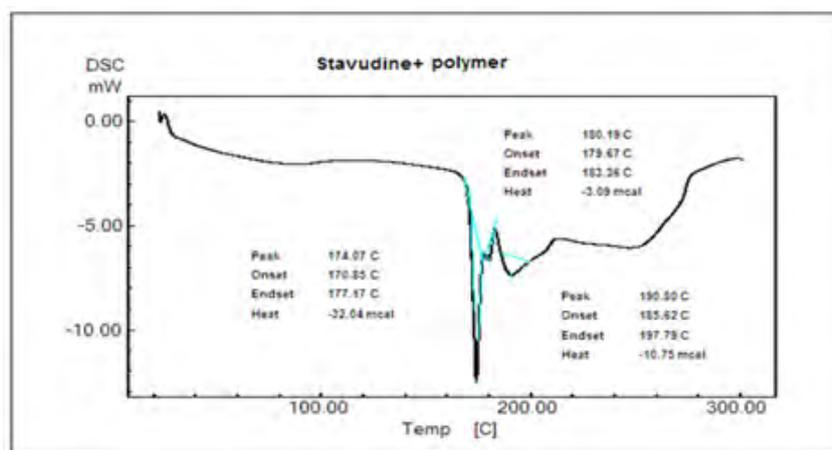
Figure no.6: DSC thermogram of Stavudine mixture
