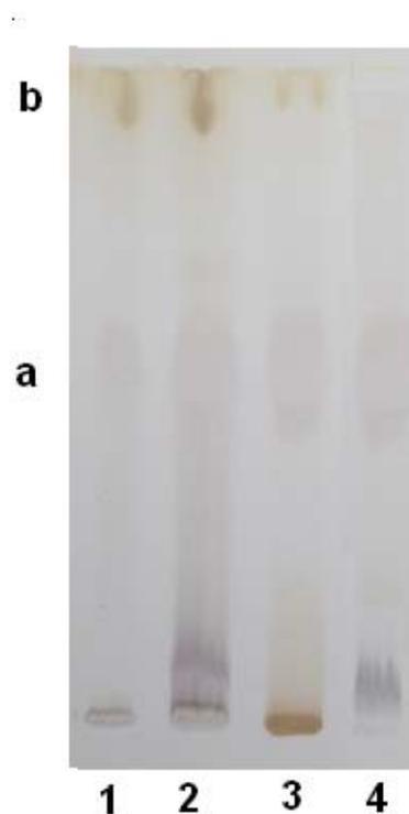
Figure 1: Image of TLC plate where 1- Petroleum ether extract 2- Solvent ether extract 3- Methanol extract 4- Isolated crude Embelin
