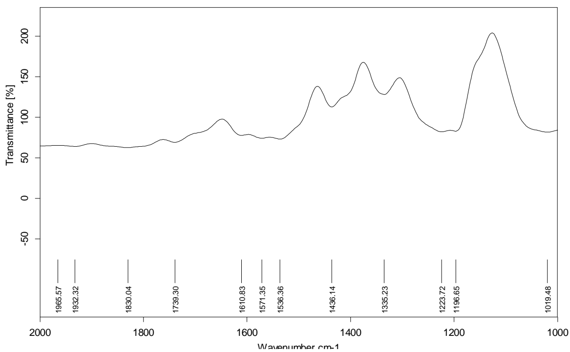
Figure 9: FTIR spectra of carbopol971P in Wavenumber 2000- 1000 cm -1
