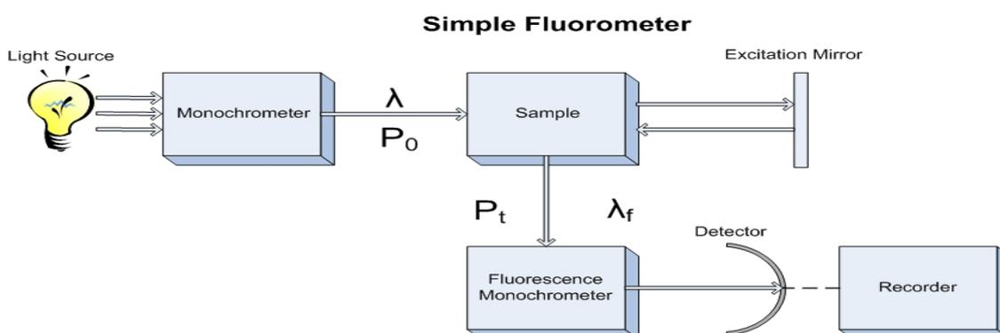
Figure 3. : Schematic diagram of Spectrofluorometer
