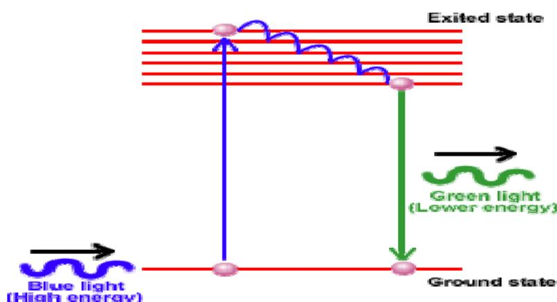
Figure 2. : Mechanism of Fluorescence.
