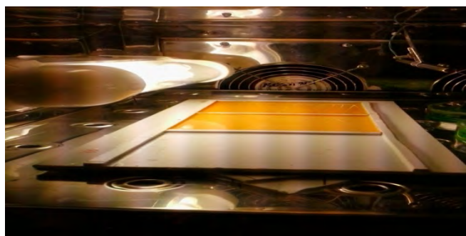
Figure 8 Lisinopril mouth dissolving film casting using Teflon mold.
