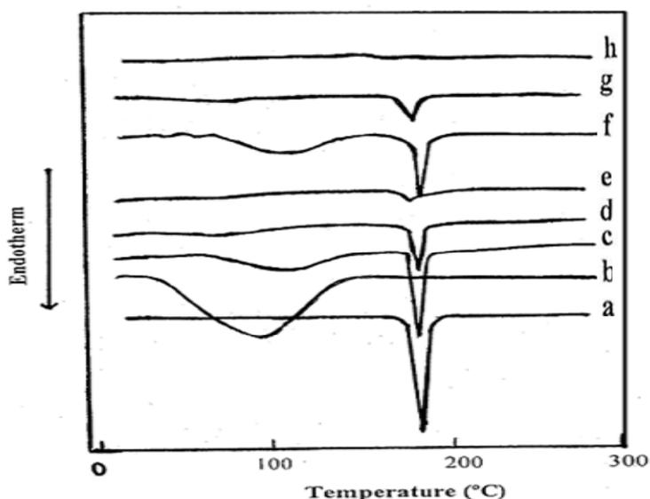
Fig.(2): DSC thermograms of different MN solid systems. Key: a) MN intact, b)  $\beta$ -CD, c) Bin-PM, d) Bin-KS, e) Bin-GS, f) Trn-PM1, g) Trn-KS1, h) Trn-GS1.
