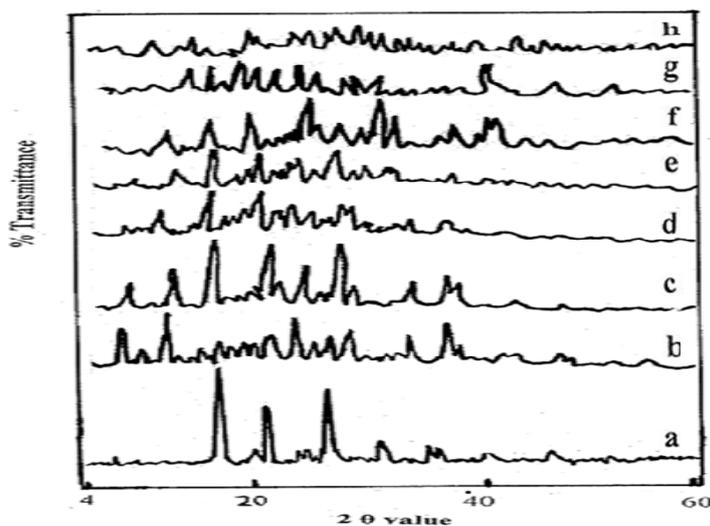
Fig.(3): XR diffractograms of different MN prepared systems. Key:a) MN intact, b)  $\beta$ -CD, c) Bin-PM, d) Bin-KS, e) Bin-GS, f) Trn-PM<sub>1</sub>, g)Trn-KS<sub>1</sub>, h) Trn-GS<sub>1</sub>.
